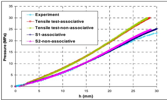
Fig. 2. Comparison between the responses of the bulge test
