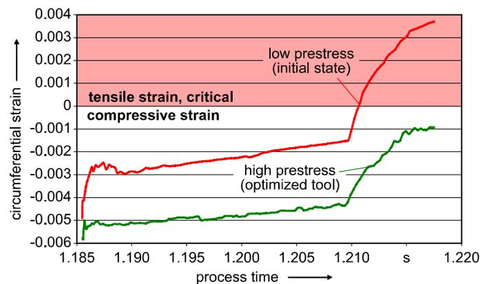
Fig. 4: Circumferential strain in the critical die area during the forging process
