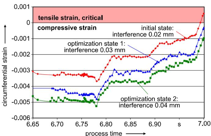
Fig. 6: Circumferential strain in the critical die area during the forging process, welding screw case study
