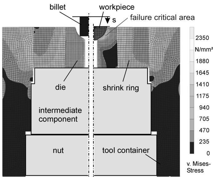
Fig. 1: FEM-model for the simulation of material flow and tool load (left: initial load, right: maximum process load)
