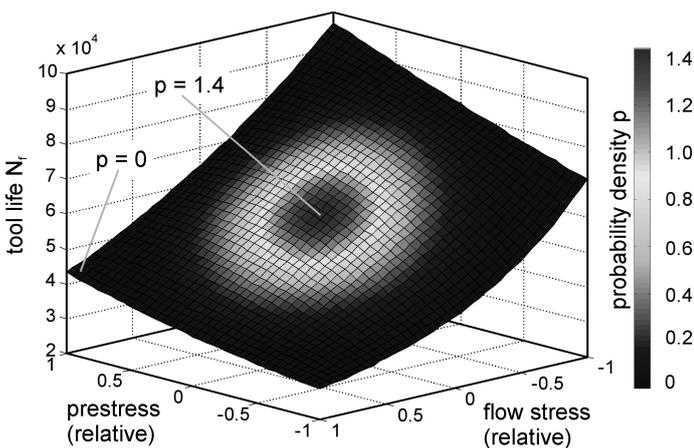
Fig. 2: Response surface of the integrated parametric statistical process model
