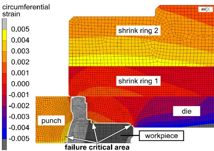
Fig. 5: FEM-model for the simulation of material flow and tool load at maximum process load (welding screw case study)
