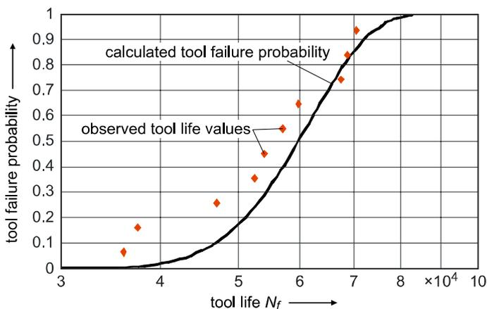
Fig. 3: Comparison of the observed tool life values in production and the calculated tool failure probability curve
