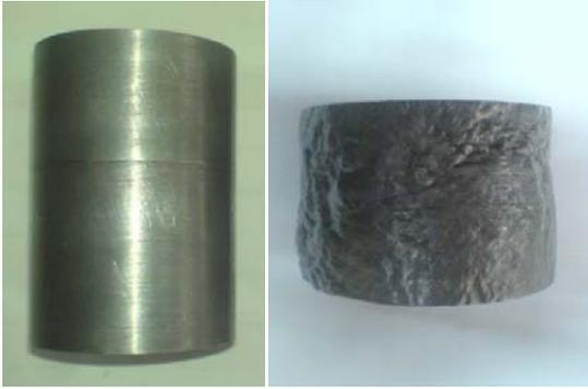
Fig. 1. Cylindrical specimen, (a) preform specimen, (b) forged specimen
