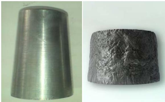
Fig. 2. Conical specimen, (a) preform specimen, (b) forged specimen.
