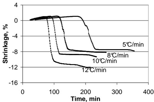
Fig 2. Shrinkage vs. time obtained at 5, 8, 10 and 12°C/min ramp temperature.
