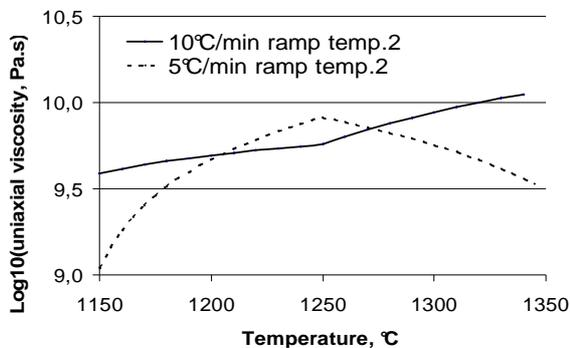
Fig 4. Uniaxial viscosity vs. temperature obtained at 5°C/min and 10°C/min ramp temperature during sintering.
