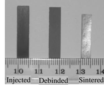
Fig 1. Injected, debinded and sintered bending test specimens realized with feedstock of powder size 5 $\mu$ m, sintering kinetic at 10°C/min.
