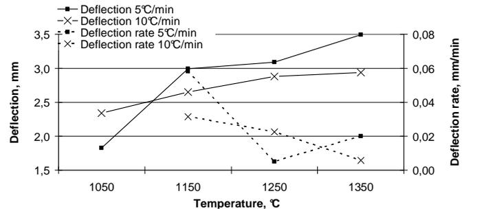
Fig 3. Deflection and deflection rate vs. time obtained at 5°C/min and 10°C/ ramp temperature.
