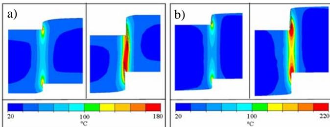
Figure 5. Temperature distribution a) without and b) with axial compression (C=2 in both cases)
