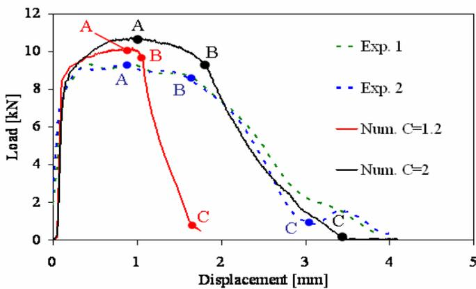
Figure 3. Load-displacement curves comparison for cropping experiments without axial compression
