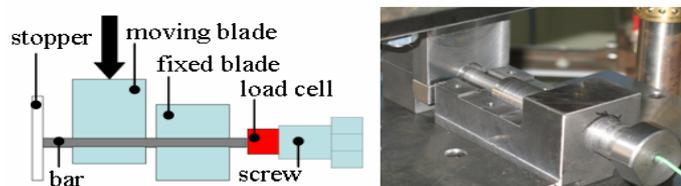
Figure 1. Cropping device: schematic illustration (left) and real setup (right)
