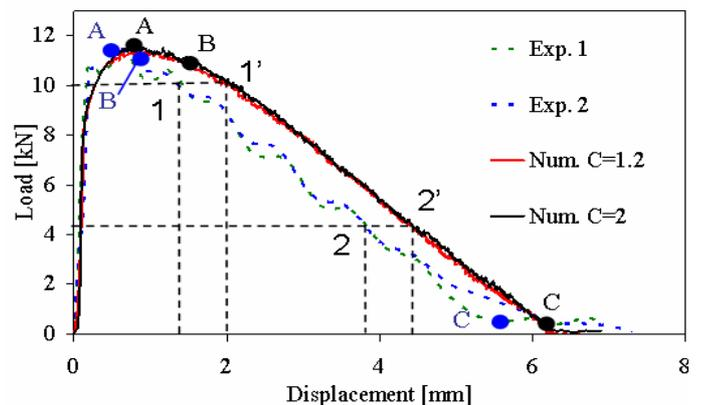
Figure 4. Load-displacement curves comparison for cropping experiments with axial compression
