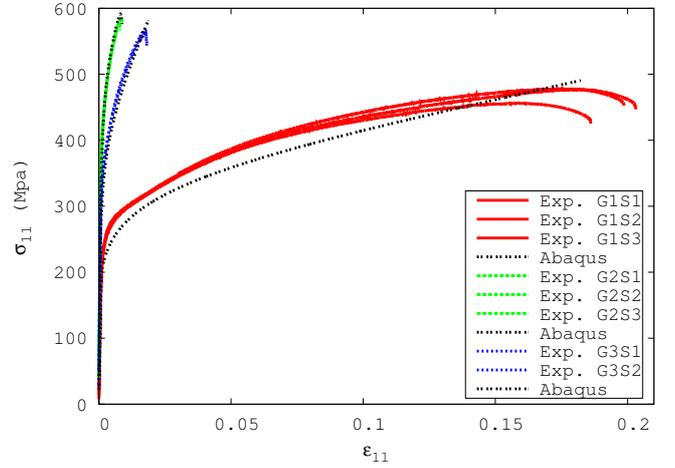
Figure 2: Comparison of the experimental identified true stress-true strain curves for microstructure M1. The parameters used in the Gurson model are given in Table 1
