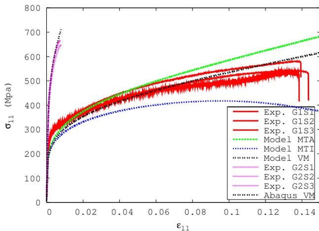
Figure 4: Comparison of the experimental and identified true stress-true strain curves for microstructure M2. Several homogenization schemes are compared for the case of G1. VM is the multi-level (recursive) homogenization scheme. MTA and MTI are the Mori-Tanaka schemes with the anisotropic and isotropic descriptions of the matrix respectively.
