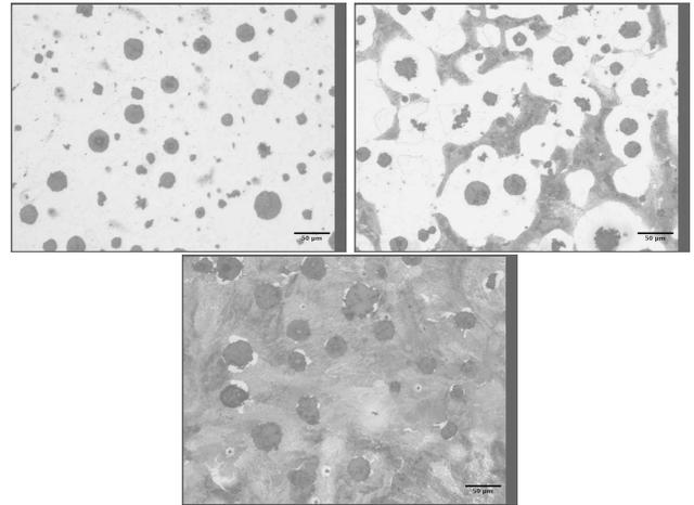
Figure 1: Picture of microstructures M1(top), M2(middle) and M3(bottom). The white and light grey zones are ferrite and pearlite respectively. The graphite nodules appear as dark disks.
