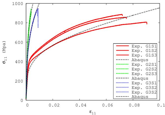
Figure 3: Comparison of the experimental and identified true stress-true strain curves for microstructure M3. The parameters used in the Ramberg-Osgood model are given in Table 1
