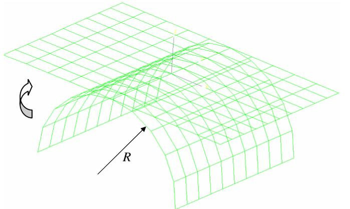
Fig 3 Blank design of a cylindrical sheet
