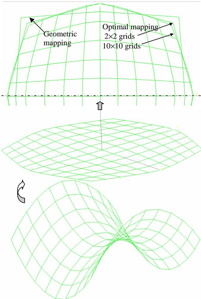
Fig 4 Blank design of a hyperbolic parabolic sheet
