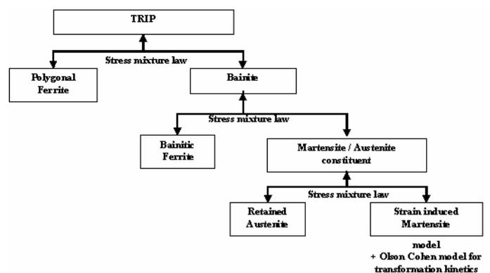
Fig. 3 - Principle of the model based on the complex TRIP microstructure decomposed into its various constituents
