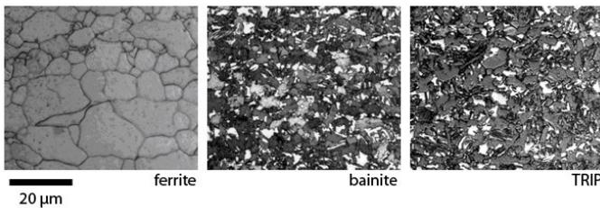
Fig. 1 - Microstructures of the different CMnAl alloys
