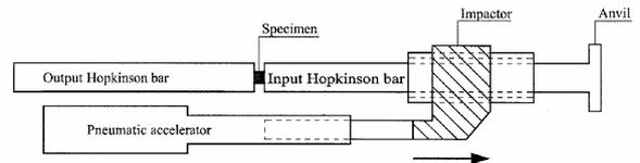
Fig. 2 - Principle of the split Hopkinson tensile bar
