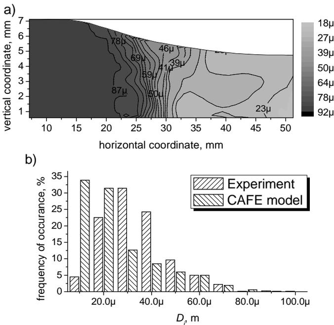
Fig. 3. Results of CAFE model,  $T = 1150^{\circ}\text{C}$ : a) distribution of average grain size [μm] at the cross section of the rolled sample, b) comparison of grain size distribution calculated by CAFE model and measured at the centre of the sample.
