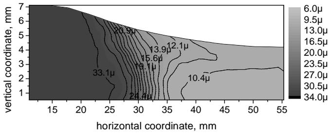
Fig. 2. Distribution of average grain size [μm] at the cross section of the rolled sample calculated by CAFE model for  $T = 950^{\circ}\text{C}$ ;
