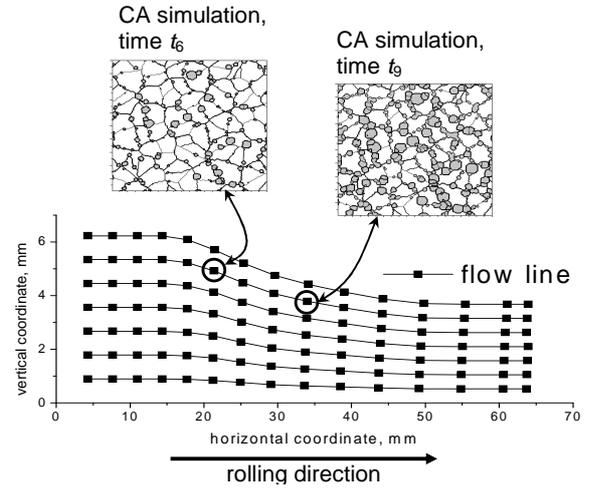
Fig. 1. The idea of the CAFE model – local values of macroscopic thermal and mechanical parameters are passed to micro-scale CA model predicting evolution of microstructure
