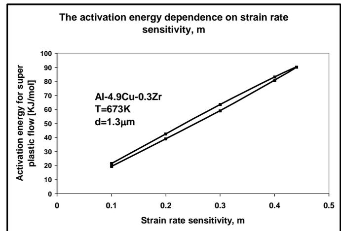
Fig. 2, Dependence of activation energy for super plastic flow of thermo mechanical worked Al-4.9Cu-0.3Zr alloy on strain rate sensitivity at 673 K, with grain size  $d = 1.3 \mu$ m.
