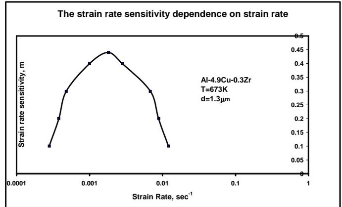
Fig. 1, Dependence of strain rate sensitivity ( $m$ ) on strain rate  $\xi_{\perp}$  of Al-4.9Cu-0.3Zr alloy at 673 K, with grain size  $d = 1.3 \mu$ m. Information obtained from reference [10].
