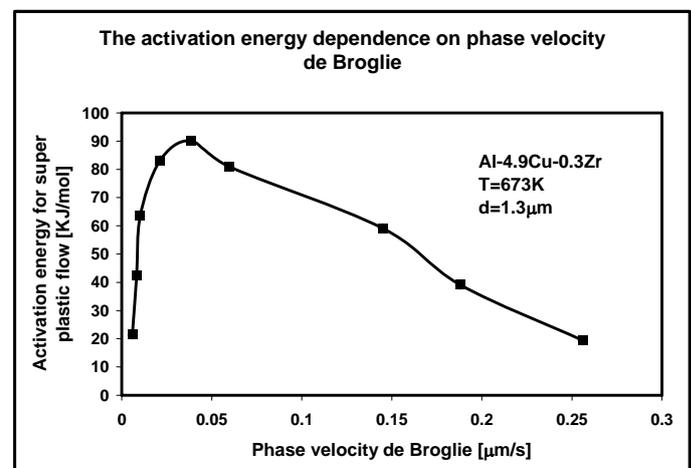
Fig. 3, Dependence of activation energy for super plastic flow of thermo mechanical worked Al-4.9Cu-0.3Zr alloy on velocity of phase de Broglie at 673 K, with grain size  $d = 1.3 \mu$ m.
