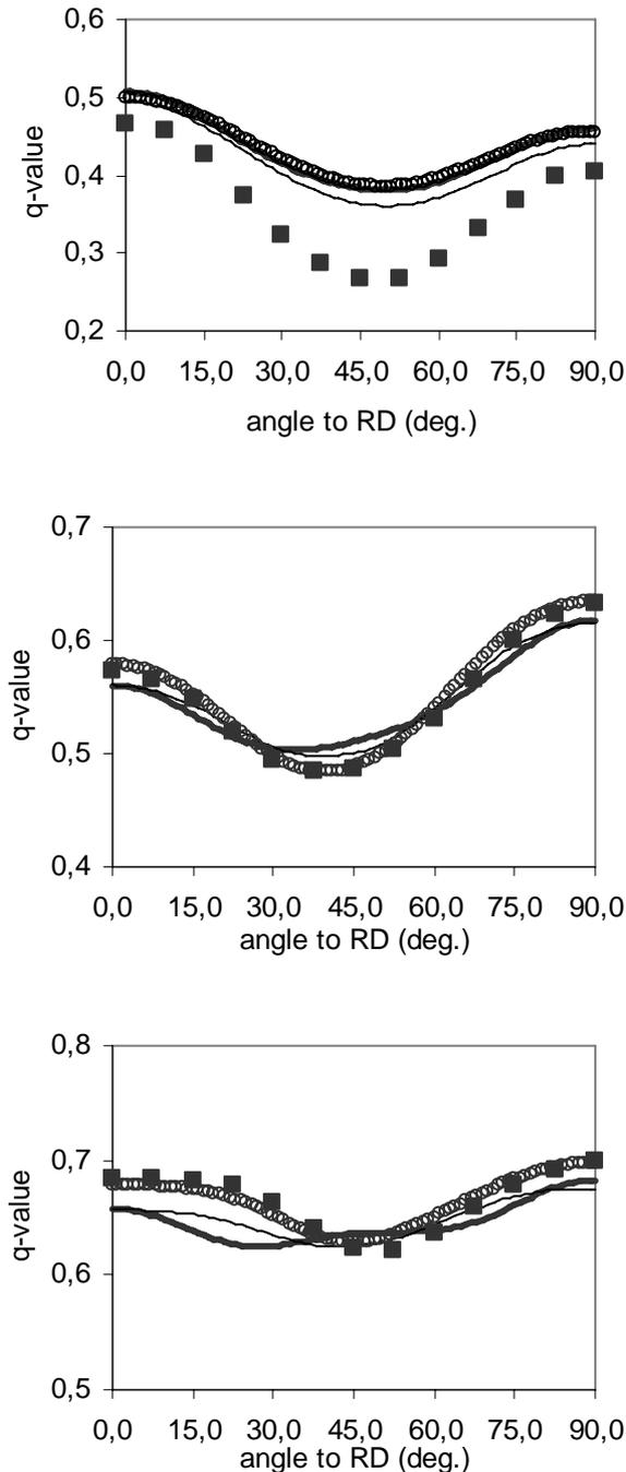
Fig. 1:  $q$ -values in function of the angle to the rolling direction for (a) Aluminium 6016-T4 alloy (T.I. 2.31); (b) Low carbon steel (T.I. 1.85); (c) IF steel (T.I. 4.84). Open dots: Quantic method. Thin lines: Facet method in strain rate space. Thick lines: Facet method in stress space. Filled squares: direct Taylor results.
