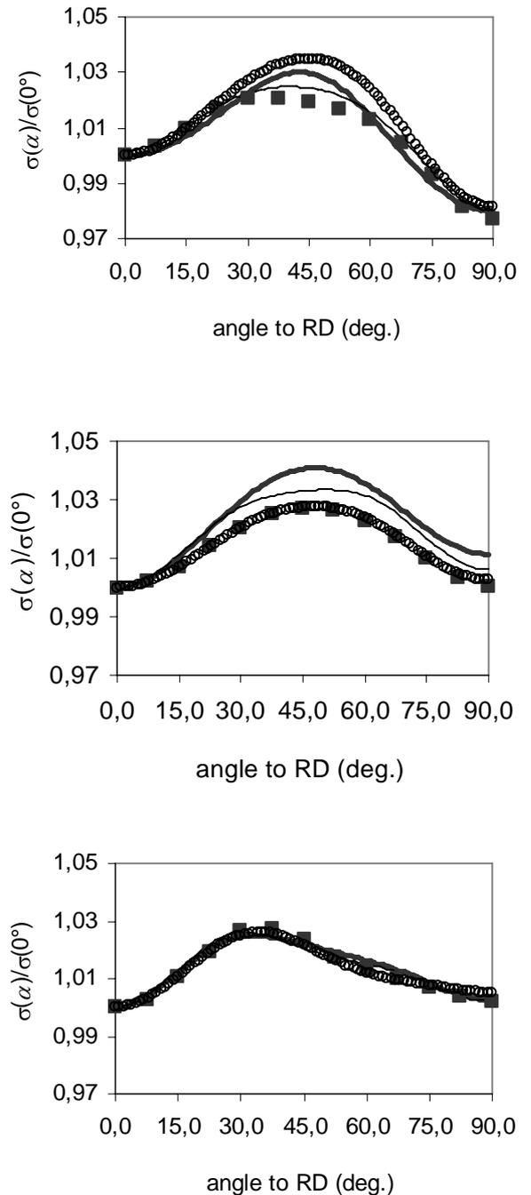
Fig. 2: Normalised yield stresses in function of the angle to the rolling direction for (a) Aluminium 6016-T4 alloy (T.I. 2.31); (b) Low carbon steel (T.I. 1.85); (c) IF steel (T.I. 4.84). Open dots: Quantic method. Thin lines: Facet method in strain rate space. Thick lines: Facet method in stress space. Filled squares: direct Taylor results.
