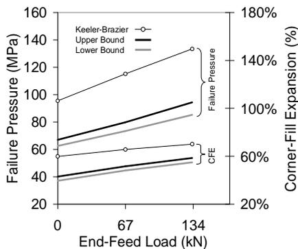
Figure 8: Predicted failure pressure and CFE vs. EF load straight tube hydroforming.
