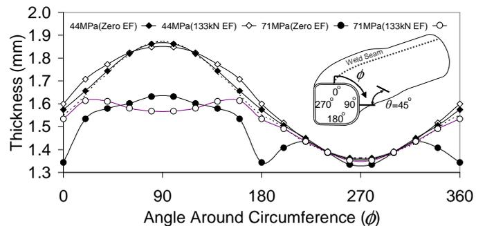
Figure 10: Pre-bent tube thickness around circumference.
