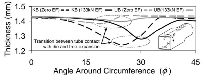
Figure 9: Straight tube thickness around circumference.
