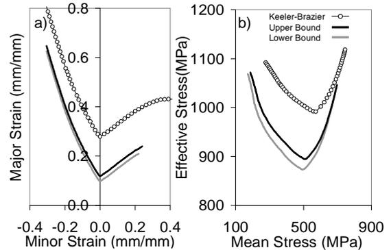
Figure 5: DP780 a) Strain based (eng) FLC's and b) XSFLC's.
