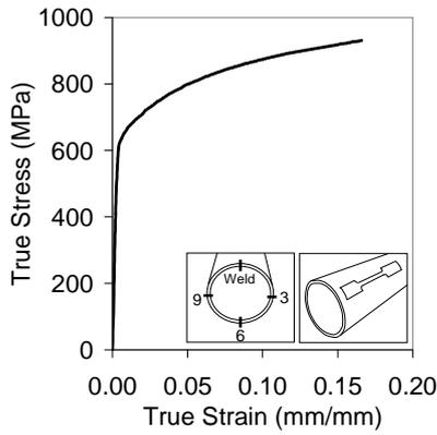
Figure 1: DP780 stress vs. strain (true) curve.
