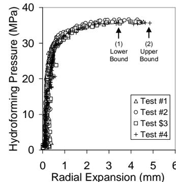
Figure 6: DP780 free-expansion burst test results.
