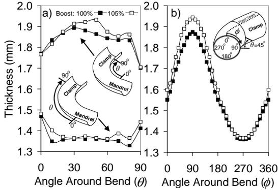
Figure 7: Thickness distribution around a) inside and outside of the bend b)  $360^\circ$  around the circumference of the bend.
