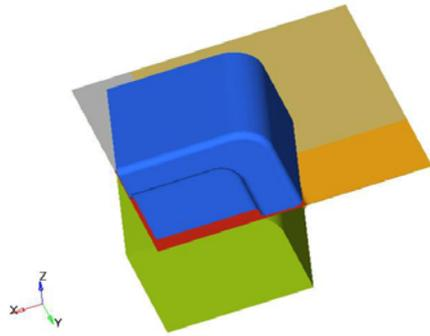
Fig. 4. FE Model created for the sheet hydroforming process simulation
