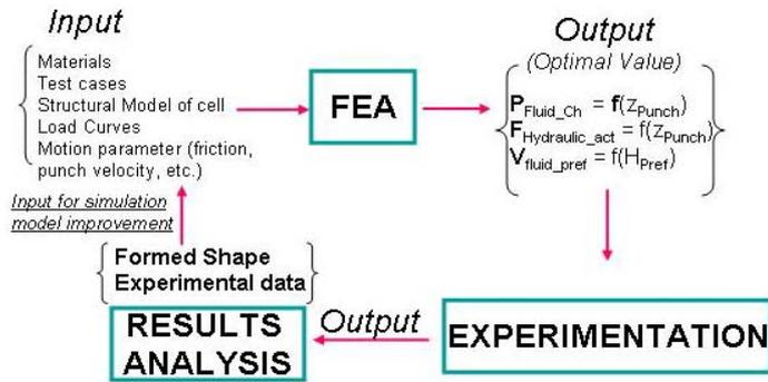
Fig. 10. The numerical – experimental correlation phase
