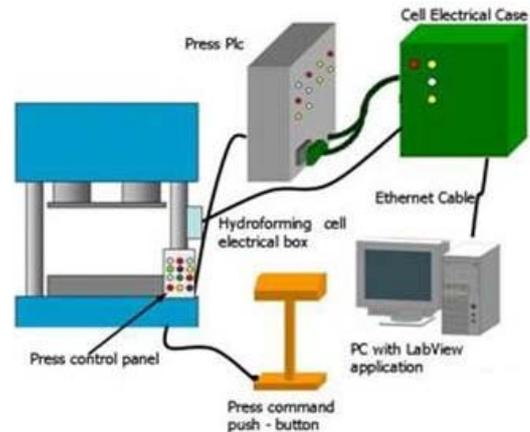
Fig. 8. Scheme of Communication
