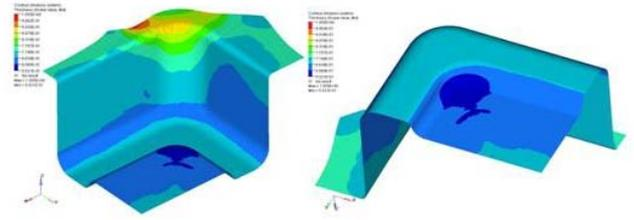
Fig. 12. Thickness distribution
