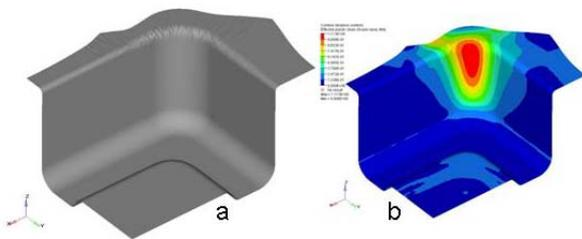
Fig. 11. (a) Fe Model; (b) Effective Plastic strain at the end of the die stroke
