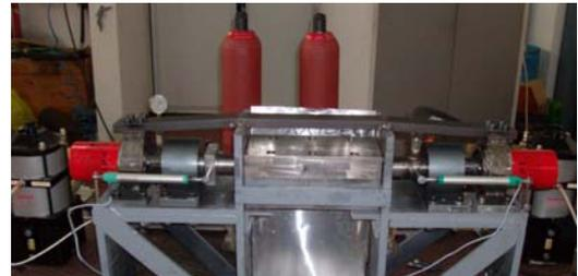
Figure 3: T tube hydroforming equipment.
