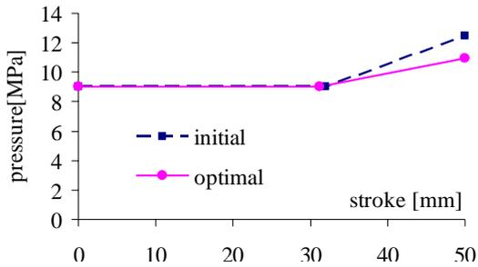
Figure 5: Initial and optimal pressure curves (thickness: 1mm).
