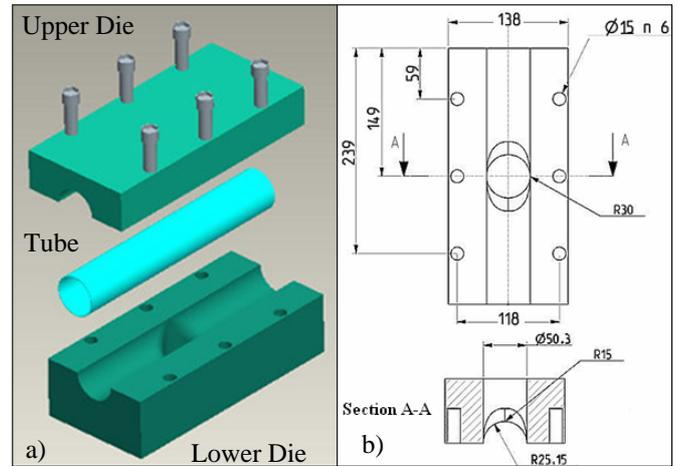
Figure 1: a) tube and dies; b) lower die dimensions.
