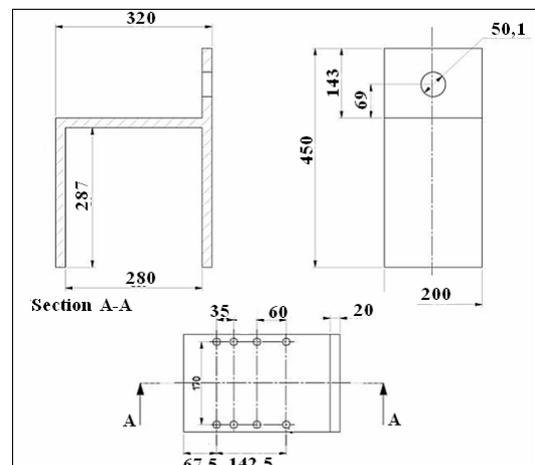
Figure 4: Equipment frame dimensions.
