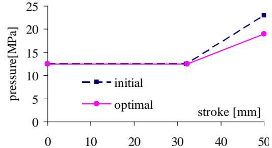
Figure 7: Initial and optimal pressure curves (thickness: 1.5mm).
