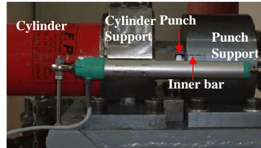
Figure 2: The axial push unit.
