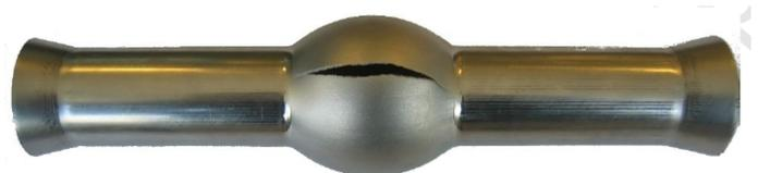
Figure 6: Bulged tube with bursting
