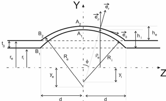
Figure 3: Geometric configuration for tube bulging
