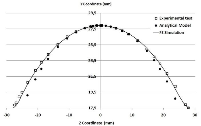
Figure 9: Experimental, analytical and numerical bulge profile
