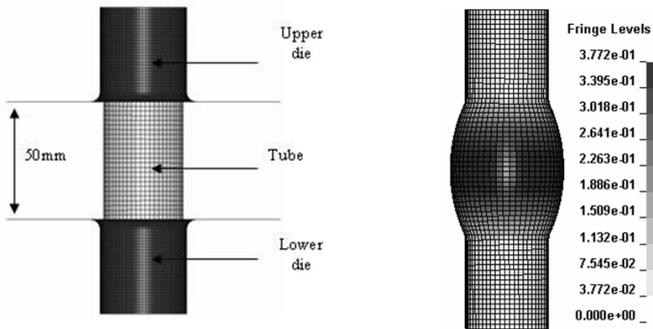
Figure 4: Finite element modelling and strain distribution on the tube
