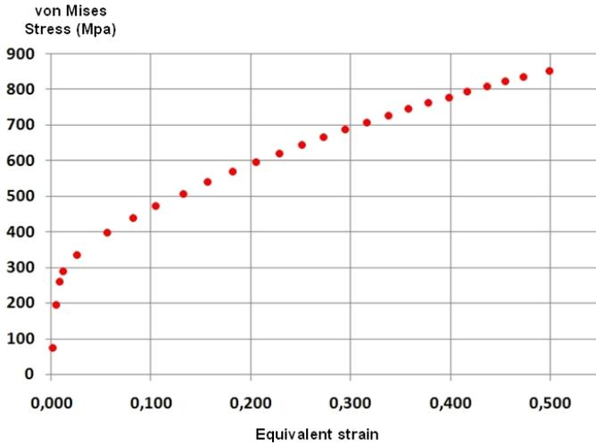
Figure 7: Experimental tube hardening law
