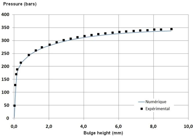
Figure 8: Experimental and numerical pressure variation with bulge height
