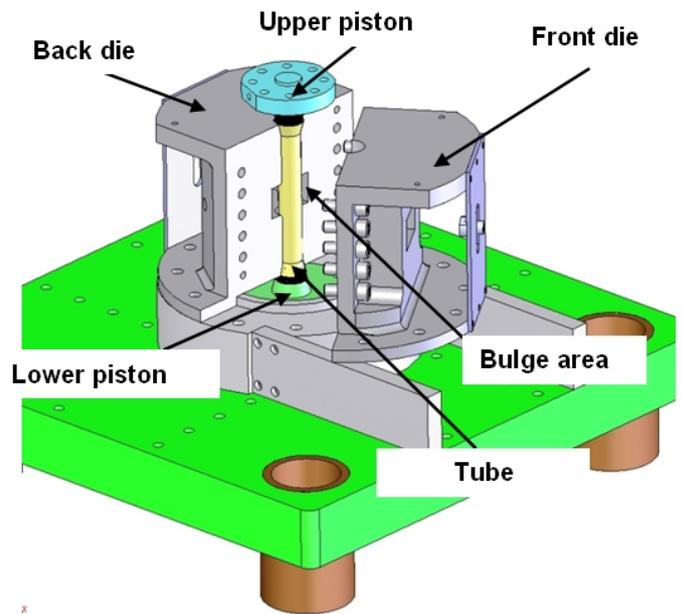
Figure 1: Experimental device for tube bulging tests
