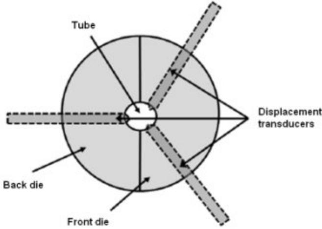
Figure 2: Displacement transducers positioning
