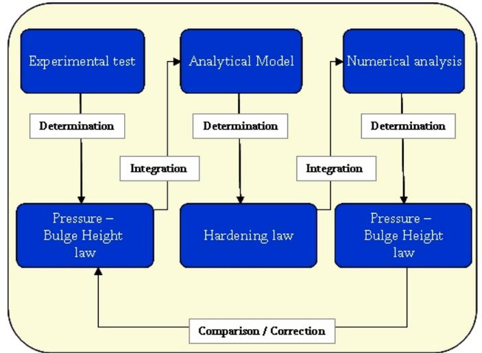
Figure 5: Methodology to determine and evaluate a tube hardening law
