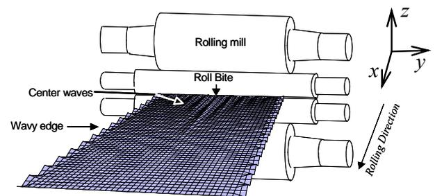
Figure 1. Schematic illustration of flatness defects [1].
