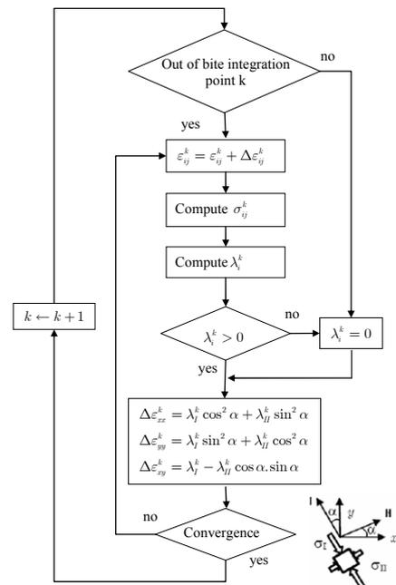
Figure 5. Algorithm of coupling Lam3/tec3 with a steady state simple buckling model:  $\epsilon_{ij}$  and  $\sigma_{ij}$  are respectively the strain increment tensor and the stress components,  $\alpha$  defines the principal directions  $I$  and  $II$  in the laboratory reference frame.
