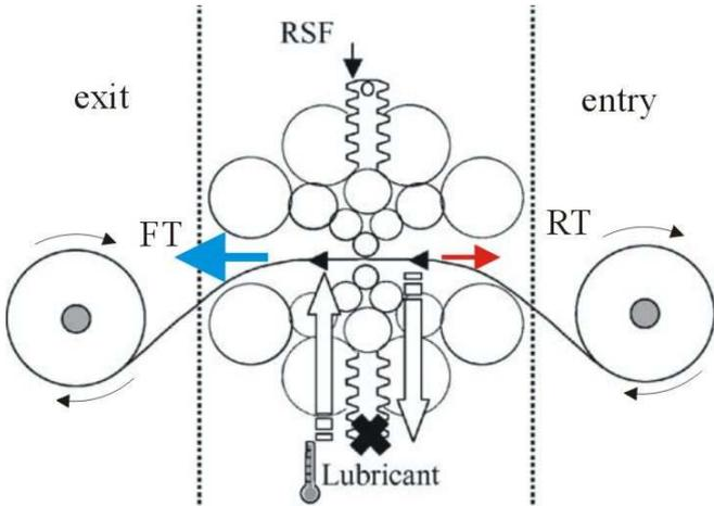
Fig. 1. Overview of a Sendzimir type mill
