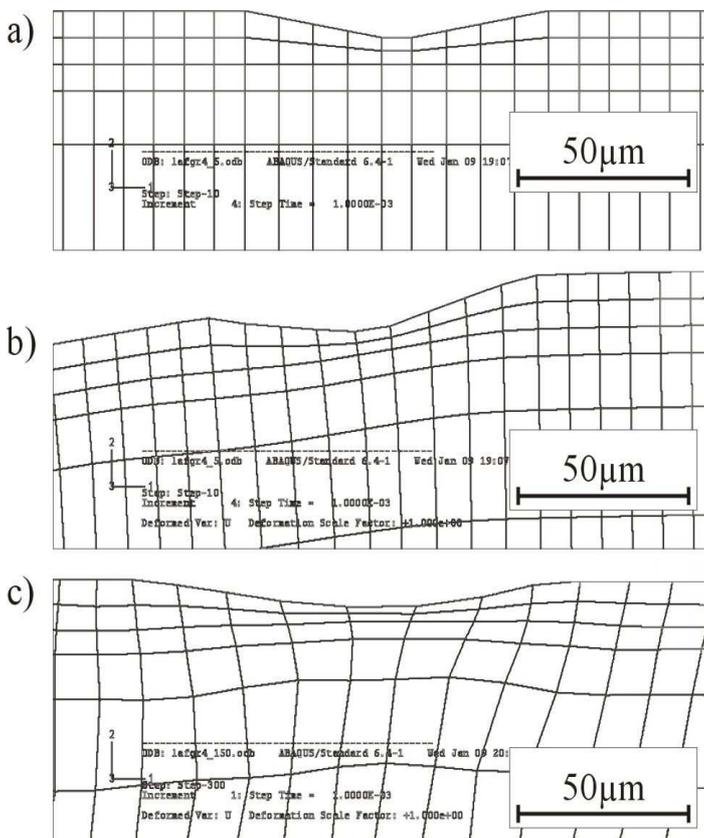
Figure 4. a) initial asperity mesh b) deformed mesh at roll bite entry c) deformed mesh at roll bite exit
