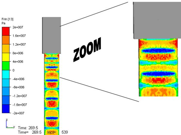
Fig. 2 : Pressure field in the secondary cooling zone
