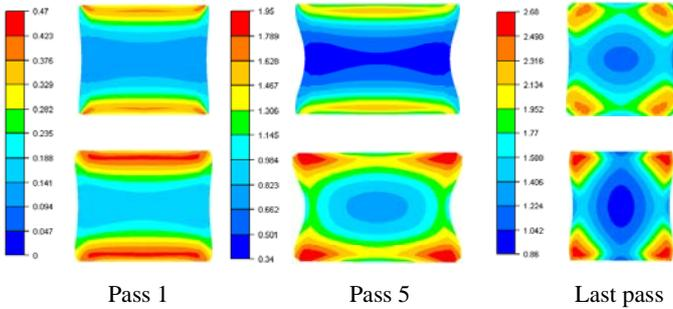
Fig. 5 : Cumulated strain evolution during rolling for two roll pass design leading to the same final section (LAM3®)
