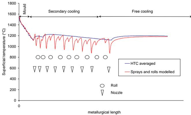
Fig. 1 : Temperature evolution : primary and secondary cooling zones
