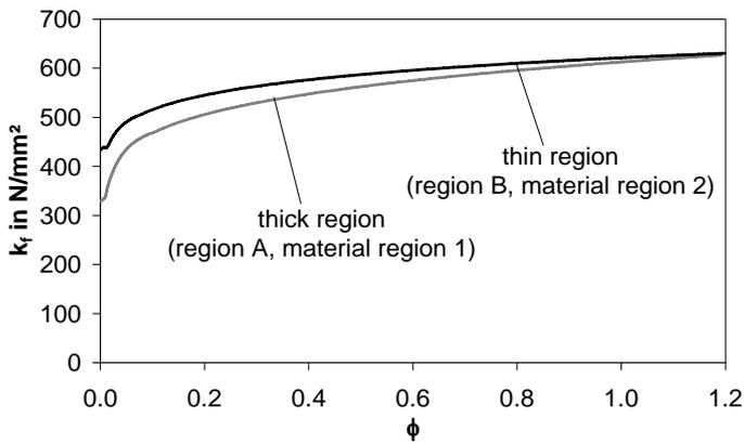
Fig. 10. Extrapolated yield curves obtained by tensile tests
