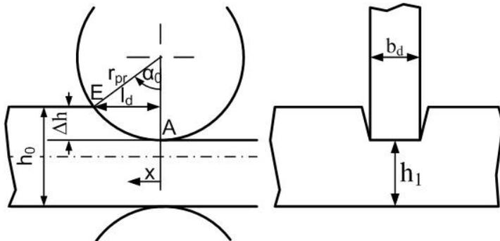
Fig. 3. Roll gap geometry in Strip Profile Rolling (SPR) left: longitudinal section, right: cross section [4]
