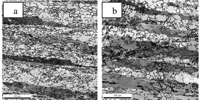
Figure 3: Subgrain structure analysis by EBSD. Low angle boundaries in black, high angle boundaries in white. Initial rolling temperature of a)  $550^\circ\text{C}$  and b)  $580^\circ\text{C}$
