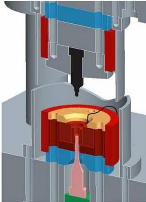
Fig. 4 Thermal system for a warm forming micro tool-set
