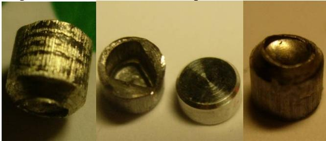
Fig. 7 Left: Formed component at 20°C with cracks in the skirt
