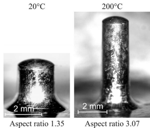
Fig. 4. Temperature effect on the aspect ratio pin diameter 2.0 mm
