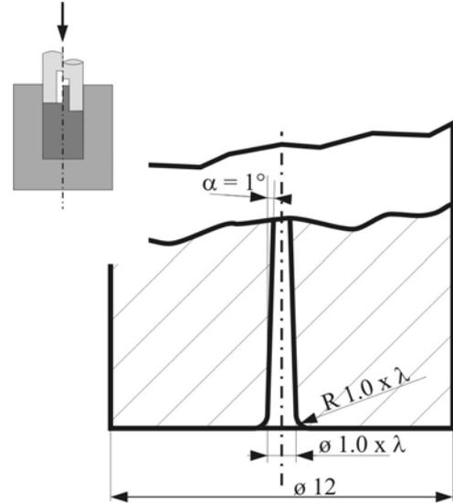
Fig. 2. Geometrical dimensions of the punch
