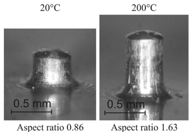
Fig. 5. Temperature effect on the aspect ratio pin diameter 0.5 mm
