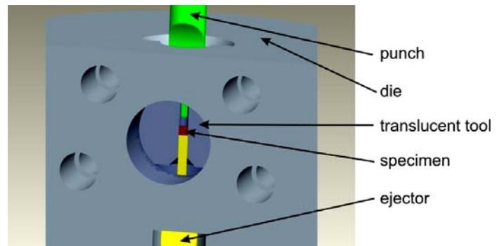
Fig. 5. Setup of the novel tool concept.
