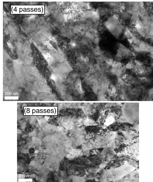
Fig. 3. Structure of copper subjected to forward extrusion followed by 4 and 8 passes of ECAP at room temperature.
