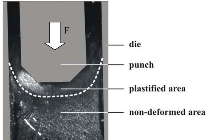
Fig. 7. Local deformation during backward extrusion of an NC\_8 UFG copper can.
