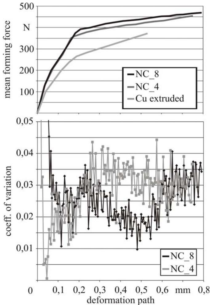
Fig. 6. Forming force and process scatter during backward extrusion of a UFG copper can.
