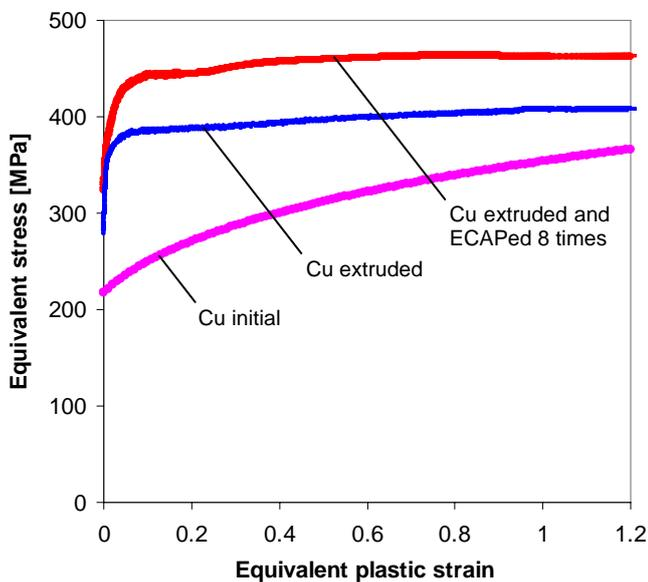
Fig. 4. Strain hardening curves for copper before extrusion, after extrusion and after extrusion and 8 passes of ECAP.
