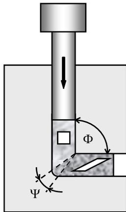
Fig. 1. Schematics of ECAP.
