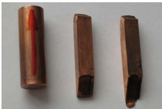
Fig. 2. Forward extruded copper bar and square samples processed by 4 and 8 passes of ECAP.
