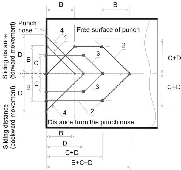
Fig. 4. The SDDG based on B, C, D; curves for 4 types of contact are shown: 1 – cutting zone, 2- ductile zone, 3 – fracture zone, 4 – die zone
