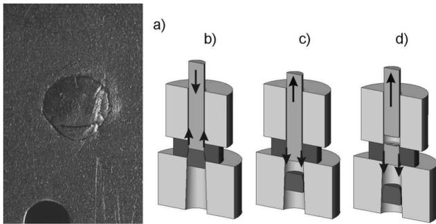
Fig. 1. Damage of the punch in micro-blanking of stainless steel 304,  $d=1$ ,  $d/h = 0.7$ : a) punch-end that remained in the strip; b), c), d) process phases (arrows show forces acting on the punch)
