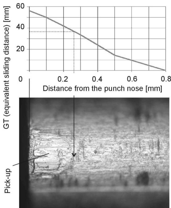
Fig. 7. Galling tendency distribution for 120 strokes and the corresponding punch picture – arrow shows the end of pick-up
