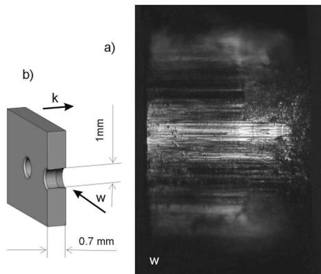
Fig. 2. Pick-ups remained on the internal surface of micro-blanked strip (a), b) specimen preparation method,  $w$  – picture direction
