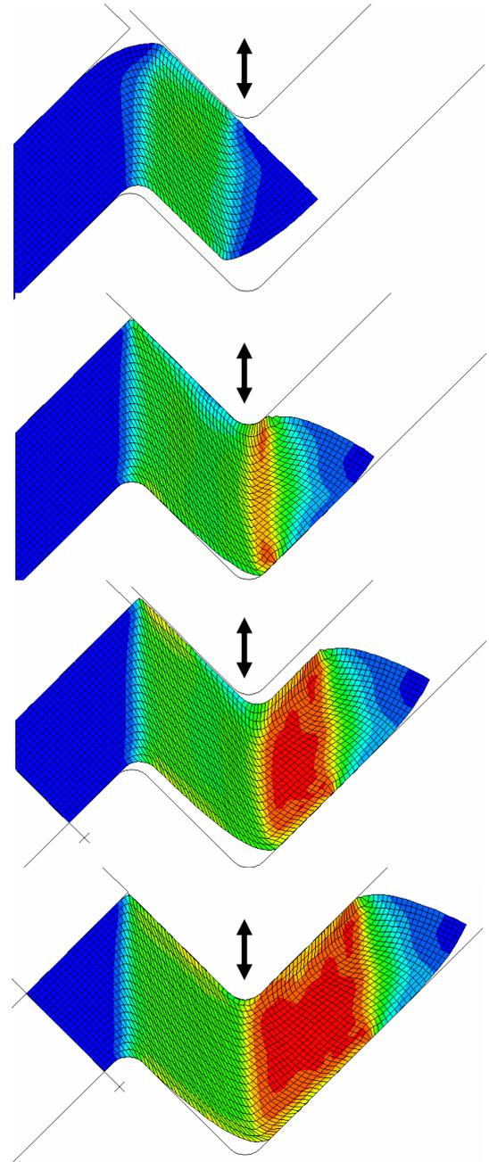
Fig. 4. Equivalent strain distribution in two-turn I-ECAP.
