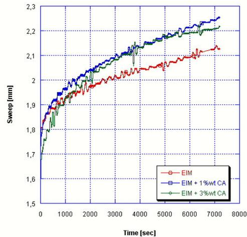
Fig. 5. Effect of CA additions on the creep behaviour of extruded + injection moulded Grivory GV5H samples
