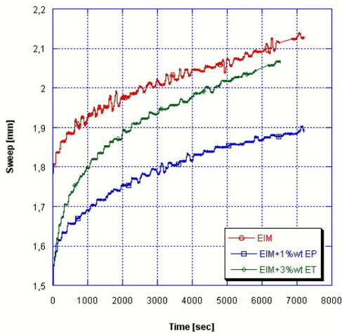
Fig. 4. Effect of EP additions on the creep behaviour of extruded and injection moulded Grivory GV5H samples
