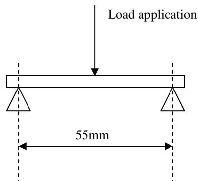
Fig. 2. Experimental setup for creep tests
