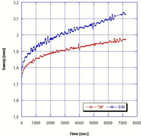
Fig. 3. Creep test results of injection moulded (IM) and extruded + injection moulded (EIM) Grivory GV5H samples
