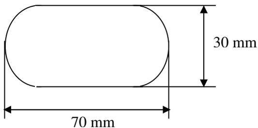
Fig. 1. Injection moulded 2 mm thick samples
