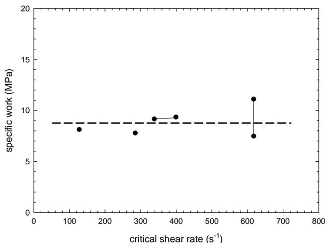
Figure 5. Specific work versus measured critical shear rates required for the formation of shish-kebabs in the sheared PB0400 ( $\gamma=100$ ). The dashed line corresponding to the critical specific work is added for clarity.
