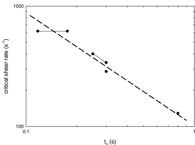
Figure 4. Measured critical shear rates required for the formation of shish-kebabs versus shearing time for the flow-induced crystallization of PB0400 ( $\gamma=100$ ). The dashed line is added for clarity.
