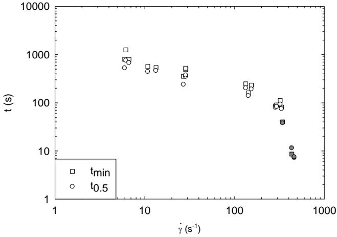
Figure 2. Characteristic time scales as a function of shear rate for the crystallization of PB0400 ( $T_c=98^\circ\text{C}$  and  $\dot{\gamma}=100$ ). The presence of the characteristic upturn in the flow birefringence is indicated by grey symbols.
