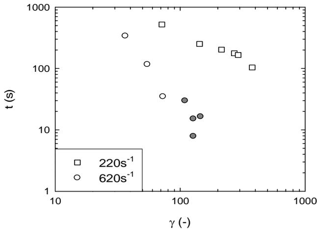
Figure 3. Crystallization time  $t_{0.5}$  of PB0400 as a function of shear strain for two different shear rates ( $T_c=103^\circ\text{C}$ ). The presence of the characteristic upturn in the flow birefringence is indicated by grey symbols.
