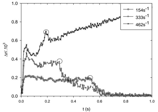
Figure 1. Flow birefringence of PB0400 ( $T_c=98^\circ\text{C}$  and  $\gamma=100$ ). Circles indicate the end of each shear pulse.
