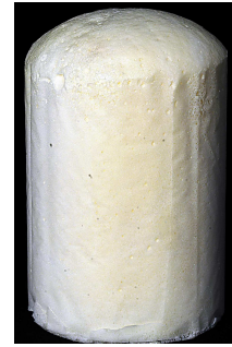
Fig. 3. Photograph of a typical foam cylinder manufactured using the RheoFoam.
