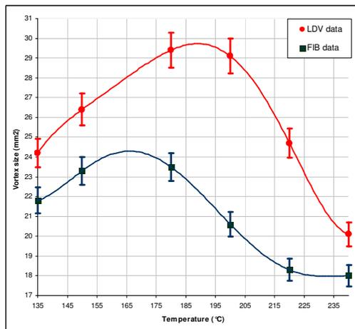
Fig. 6. Dependence of the vortex size on the temperature at  $m=0.3g/s$ , comparison between LDV and FIB data.
