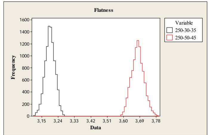
Fig. 6. Probability density functions of the top lid flatness at different process conditions
