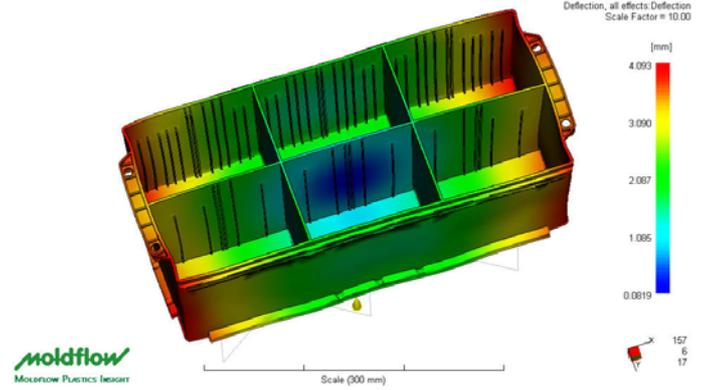
Fig. 3 Example of warpage analysis, with 10X scale factor.
