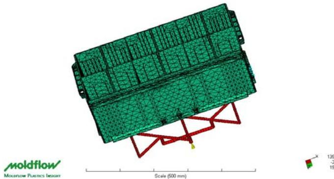
Fig. 2 Fusion mesh of the box modelled with Moldflow Plastics Insight®
