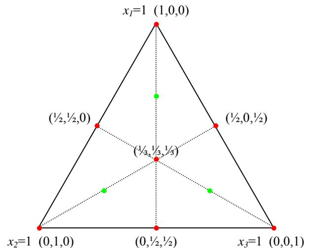
Fig. 1. Configuration of experimental runs for a  $\{3,2\}$  simplex lattice design.
