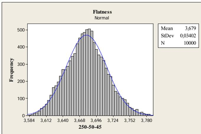
Fig. 4 Probability density functions of the top lid flatness at nominal process conditions
