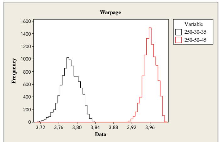
Fig. 7 Probability density functions of the longer sides warpage at different process conditions
