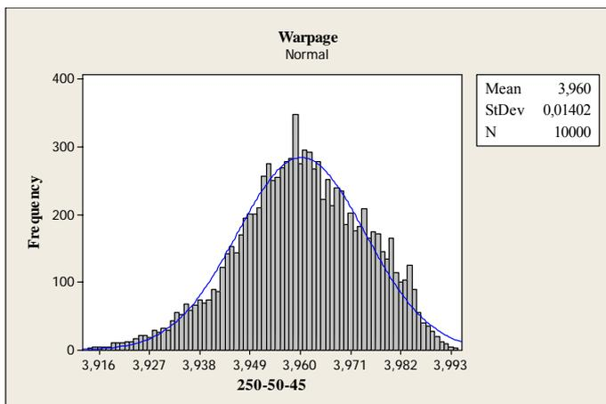
Fig. 5 Probability density functions of the longer sides warpage at nominal process conditions
