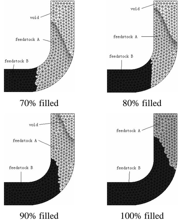
Fig. 2. Co-injection filling state
