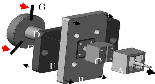
Figure 1: Ejection system – movements on the demolding stage and transfer of forces on force sensors.
