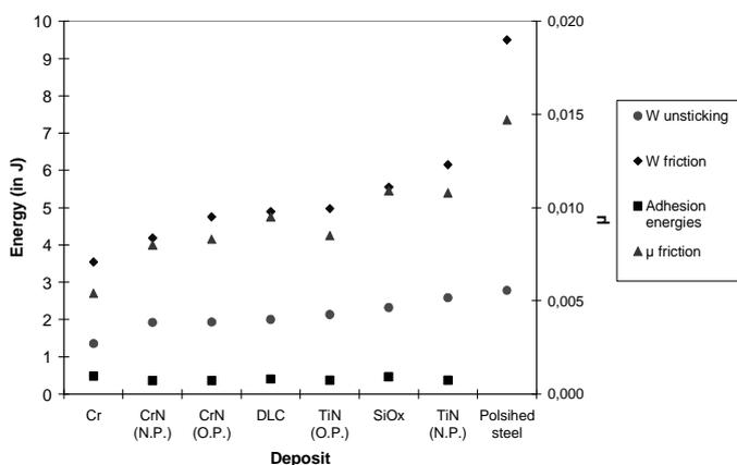
Figure 6: Comparison of the different contributions of work towards adhesion energies and friction coefficient for PBT
