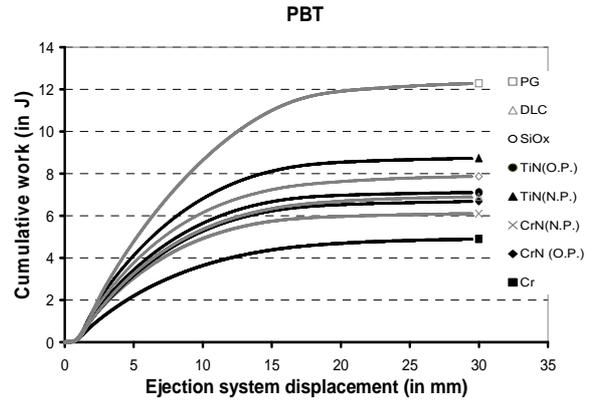
Figure 4: Evolution of cumulative ejection work for PBT
