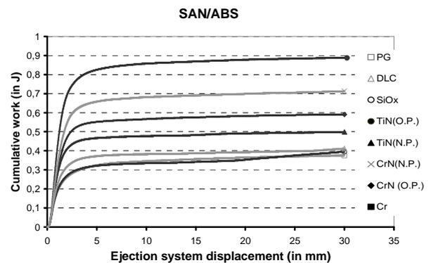
Figure 2: Evolution of cumulative ejection work for SAN/ABS
