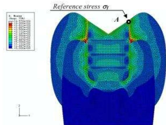
Fig. 4. Huber-Mises stress in Class I restoration
