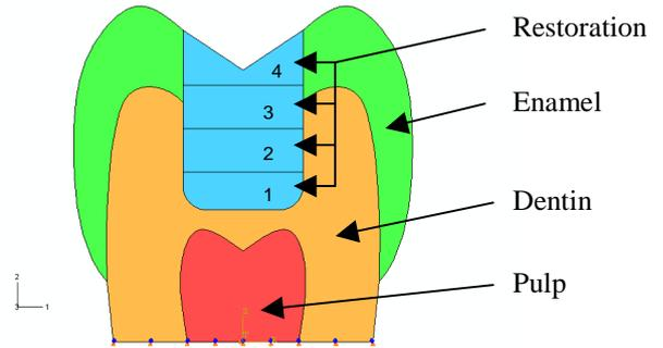
Fig. 3. Assumed tooth-restoration geometry
