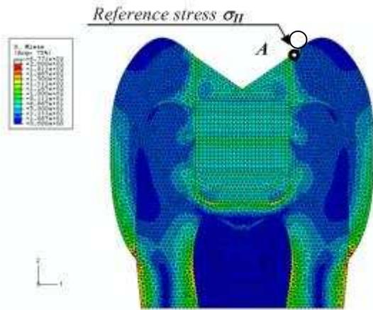
Fig. 5. Huber-Mises stress in Class II restoration
