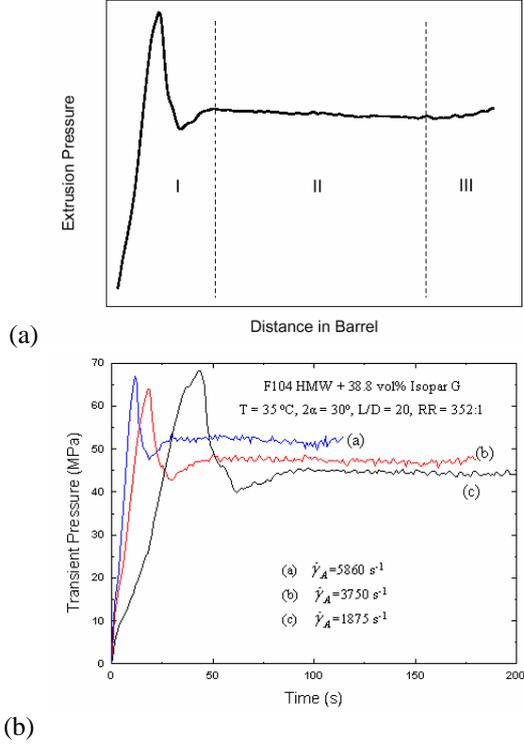
Fig. 1. PTFE paste extrusion at 35°C: (a) typical extrusion pressure vs. distance in the capillary, (b) effect of apparent shear rate  $\dot{\gamma}_A$  on pressure transient (RR=area reduction ratio)
