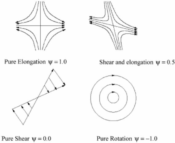
Fig. 2. Flow fields corresponding to different parameters  $\psi$
