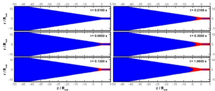
Fig. 3. Transient simulation results for the fibrillated (red) / unfibrillated (blue) regions for  $R_{res}/R=12.5$ ,  $R=0.381$  mm,  $\dot{\gamma}_A = 1390$  s<sup>-1</sup>, convergence angle  $2a=30^\circ$
