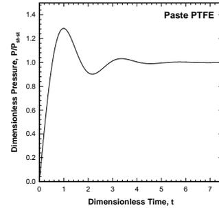
Fig. 4. Transient simulation results for the dimensionless pressure  $P/P_{st-st}$  for  $R_{res}/R=12.5$ ,  $R=0.381$  mm,  $\dot{\gamma}_A = 1390$  s<sup>-1</sup>, convergence angle  $2a=30^\circ$
