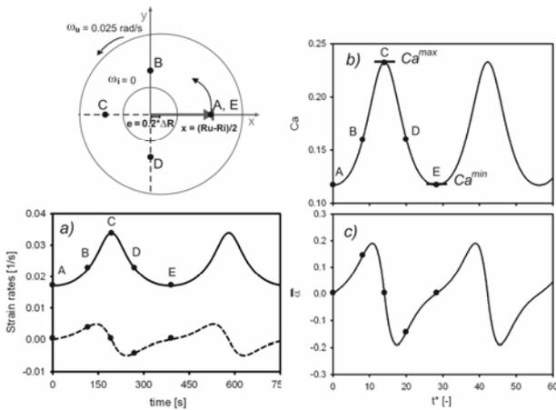
Fig. 3. Profiles for eccentric configuration with  $X = 0.2$ ,  $\omega_i = 0$  and  $\omega_o = 0.025$  rad/s along streamline starting at  $x = 30$  mm from center of the inner cylinder of: *a*) shear (—) and elongation (---) rates *b*) capillary number  $Ca$  *c*) flow type parameter  $\bar{\alpha}$ . Parts *b*) and *c*) are for a PDMS drop with initial radius of  $375 \mu\text{m}$  at a temperature of  $23^\circ\text{C}$ .
