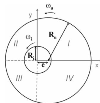
Fig. 1. Sketch of the top view of an eccentric cylinders system.
