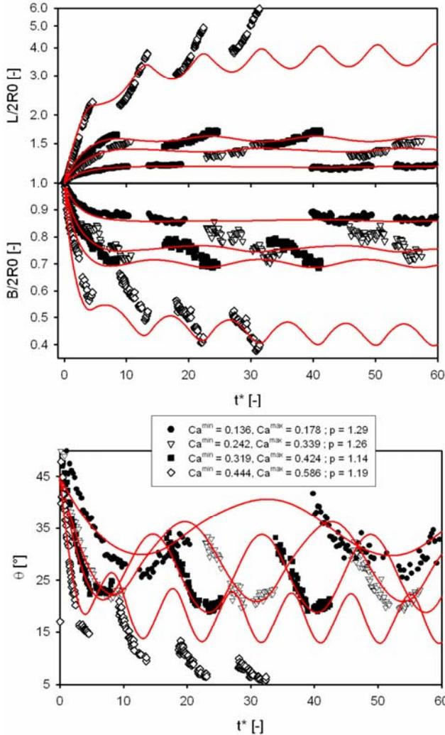
Fig. 4. Droplet deformation during sub-critical complex flows with eccentricity ratio  $X = 0.2$ ,  $\omega_1 = 0$  and variable  $\omega_2$ . Symbols represent experimental results whereas lines are predictions according to the Maffettone-Minale model.
