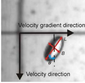
Fig. 2. Deformation parameters of a deformed droplet.
