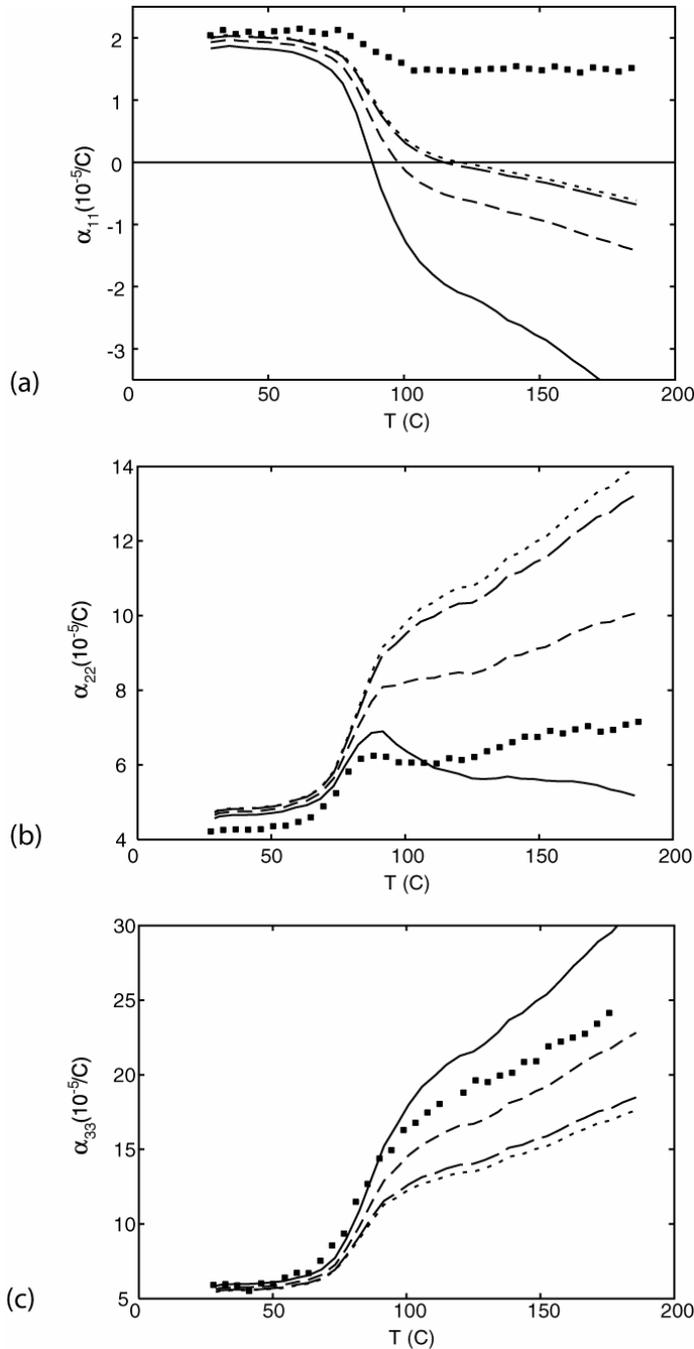
Fig. 1. Thermal expansion coefficients along the three axes of the composite: experimental values (symbols) and predictions given by the stiffness averaging procedure using the linear (unbroken line), quadratic (dotted line), and hybrid (type A: long dashes, type B: short dashes) closure approximations.
