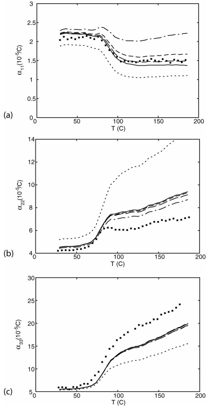
Fig. 2. Same as Figure 1, but the experimental values (symbols) are now compared to the predictions given by the stiffness averaging procedure using either the experimental fourth-order orientation tensor (unbroken line), or the closure approximations proposed by Cintra and Tucker (smooth closure: mixed dashes, fitted closure: long dashes), Chung and Kwon (short dashes), Doghri and Tinel (dotted line).
