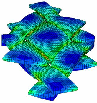
Fig. 2. Deformed unit cell. Plots of local compaction.
