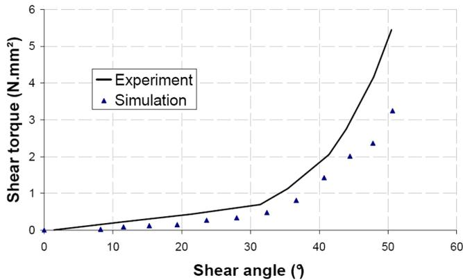
Fig. 3. Shear curve, simulation vs picture frame experiment.
