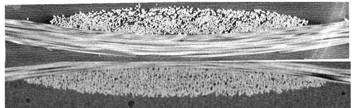
Fig. 1. Tomography reconstructed slices of a glass plain weave. Undeformed state (top) and biaxial tensioned state (bottom). (different scales)
