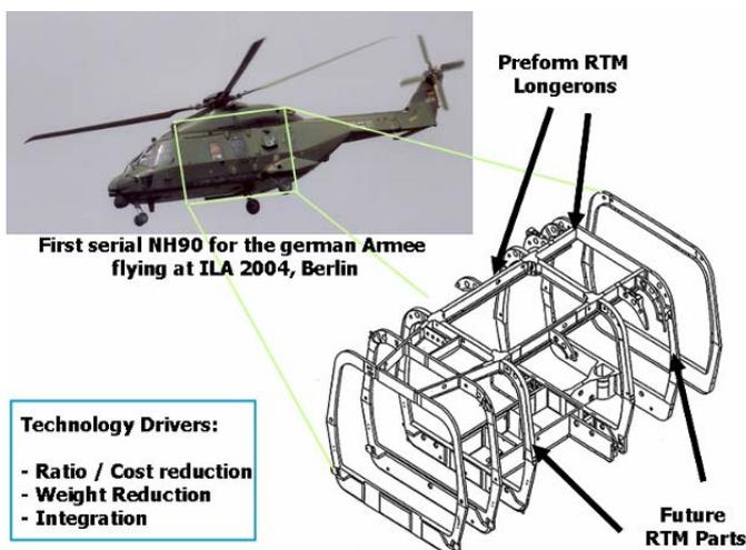
Fig. 1. Industrialisation of Preform/RTM parts in NH90
