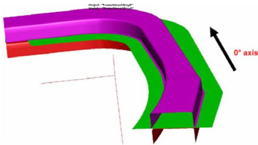
Fig. 3. Geometry of tooling and blank
