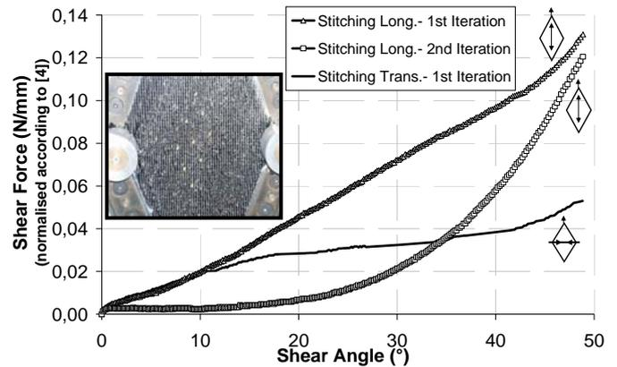
Fig.2. Trellis frame test with NCF 'A'
