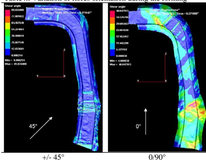
At the same time step, we notice a lower variation of angles on the material +/-45° denoting a better formability. But this forming simulation implies to consider the material as continuous. The defect types
