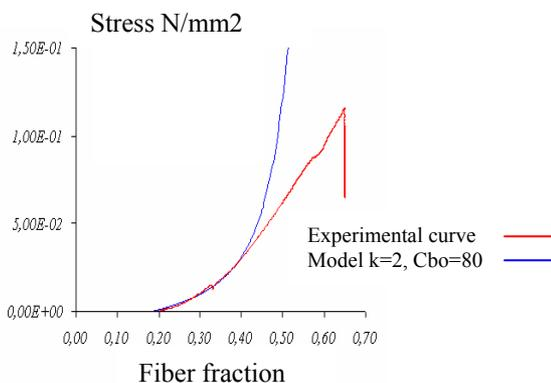
Figure 1: Validation of the model based on the equation of continuity and Darcy law for mat 624.
