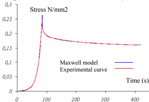
Figure 5: Validation of the rheological model of Maxwell in the case of a mate 450 of 20 plies.
