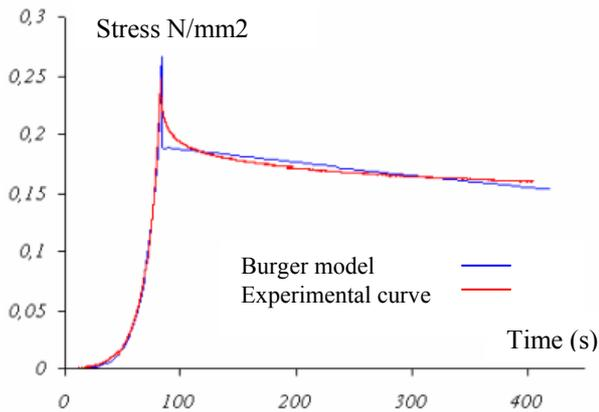
Figure 4: Validation of the rheological model of Burger in the case of a mat 450 of 20 plies.
