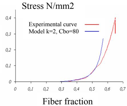
Figure 2: Validation of the model based on the equation of continuity and the Darcy's law for twill.
