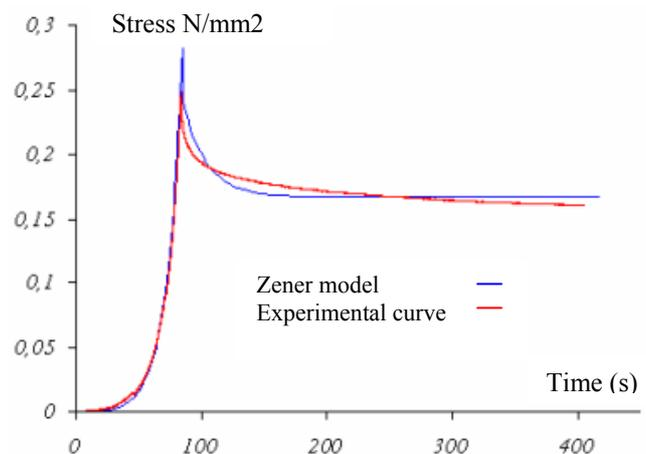
Figure 3: Validation of the rheological model of Zener in the case of a mat 450 of 20 plies.
