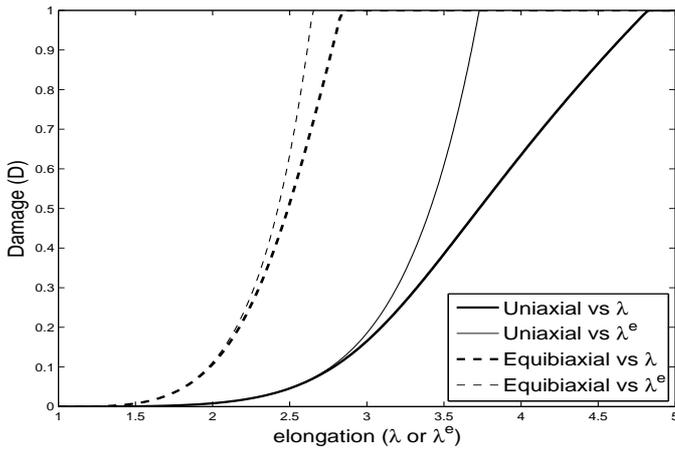
Figure 2: Damage in uniaxial and equibiaxial tests versus elongation.
