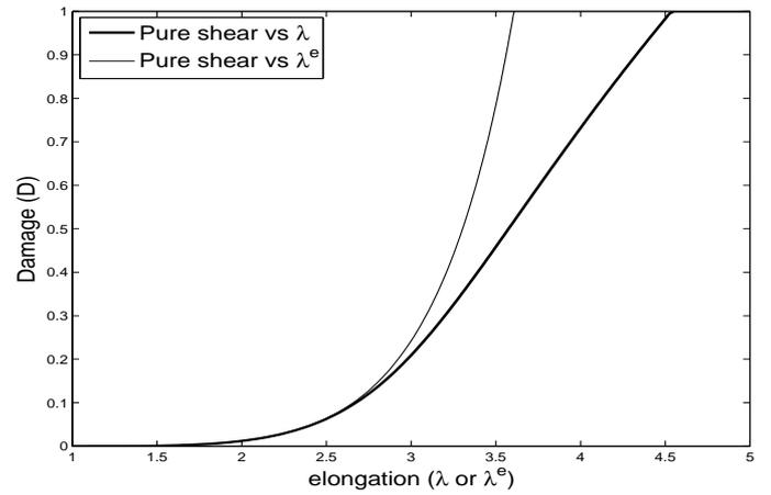
Figure 4: Damage in pure shear test versus elongation.
