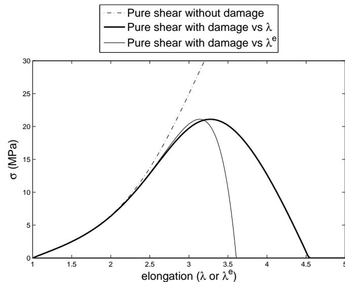
Figure 3: Stress in pure shear test versus elongation.
