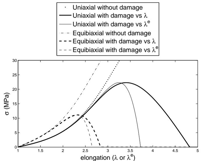
Figure 1: Stress in uniaxial and equibiaxial tests versus elongation.
