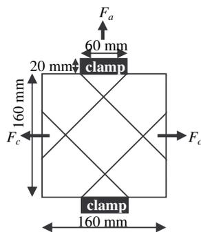
Fig 3. Specimen dimensions. The black regions indicate material underneath the clamps.  $F_a$  is the total axial force measured in the BBE tests and  $F_c$  is the transverse force applied to the specimen using a point force.
