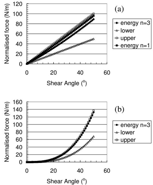
Fig 2. (a) Normalisation of a hypothetical linear force versus shear angle curve using Eqs (1), (2) and Eq (5) with  $n=1$  and 3. (b) normalisation of a cubic curve using Eqs (1) and (2) and Eq (5) with  $n=3$ .
