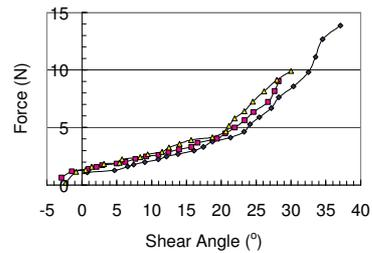
Fig 4.  $F_n$  versus shear angle for the plain weave carbon fabric before normalisation. This figure shows three repeats using the same test method.
