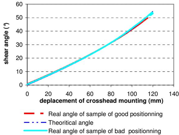
Fig1: Real angles measured by optical method of the two tests
