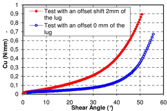
Fig2. Picture Frame test with different offset of the lug
