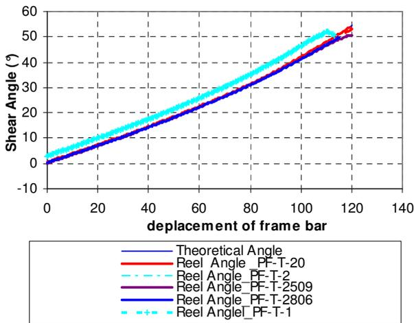
Fig 6. Offset of the initial angle between arms
