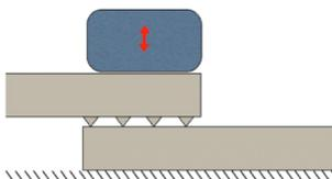
Figure 1 : Ultrasonic welding of two plates
