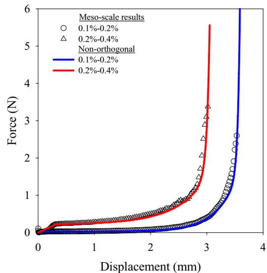
Fig. 5. Force-displacement curves for shear tests under non-even biaxial tension mode
