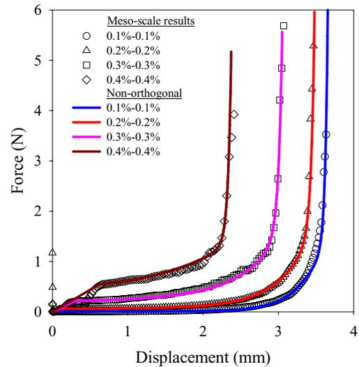
Fig. 3. Force-displacement curves for shear tests under even biaxial tension mode
