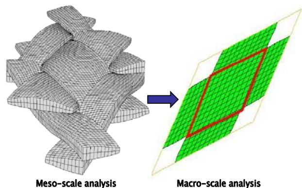
Fig. 1. Schematic description how to obtain the shear property for macro-scale simulation from the meso-scale analysis
