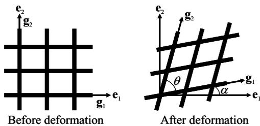
Fig. 2. Orthogonal coordinate system and non-orthogonal skew rectilinear coordinate system
