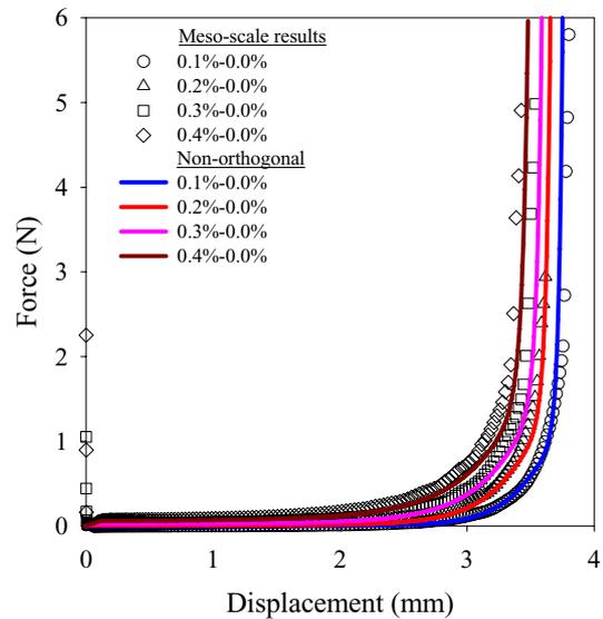
Fig. 4. Force-displacement curves for shear tests under uniaxial tension mode
