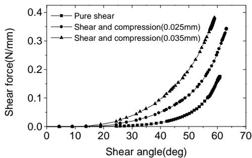
Fig.7 Interaction between compression and shear (in compression, the unit cell was compacted to 0.025mm and 0.035mm, respectively)
