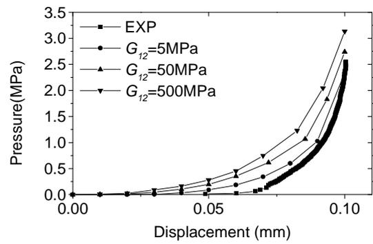
Fig.5 Comparison between experimental compaction results and FE predictions for different  $G_{12}$
