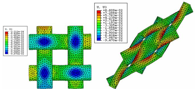
Fig.2 Predicted displacement distribution through unit cell thickness: (left) under compressive loading, (right) under pure shear loading
