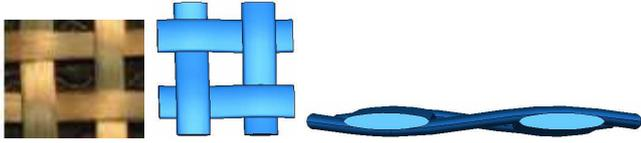
Fig.1.Chomarat 150TB (left), modelled unit cell (middle and right)
