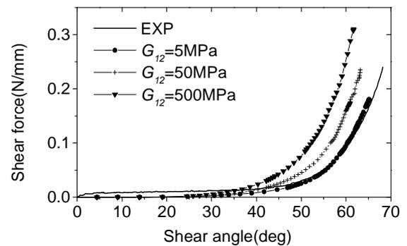
Fig.6 Comparison between experimental shear results and FE predictions for different  $G_{12}$
