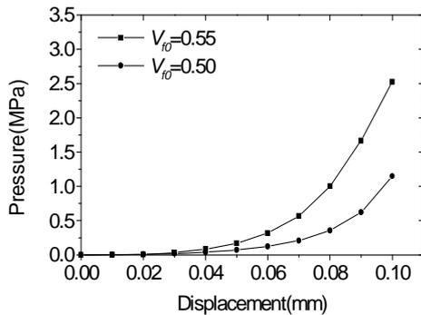
Fig.3. Effect of initial fibre volume fraction on compression
