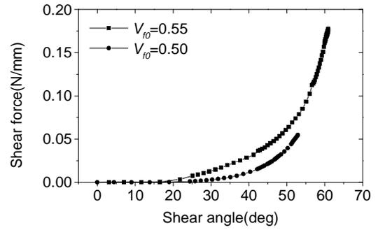
Fig.4. Effect of initial fibre volume fraction on shear
