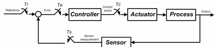
Fig.3. Closed control-loop
