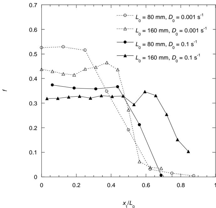
Figure 4: Evolution of the fibre content  $f$  along the normalised abscissa  $x_1/L_0$  for various initial sample lengths  $L_0$  and various strain rates  $D_0$  (compression elongation  $\lambda_f = 0.6$ ).
