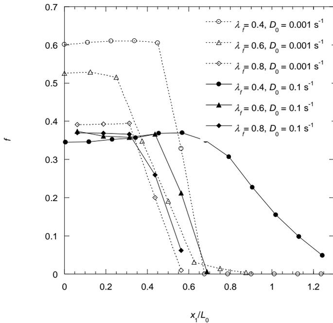
Figure 3: Evolution of the fibre content  $f$  along the normalised abscissa  $x_1/L_0$  for various compression elongations  $\lambda_f$  and various strain rates  $D_0$  (initial sample length  $L_0 = 80$  mm).
