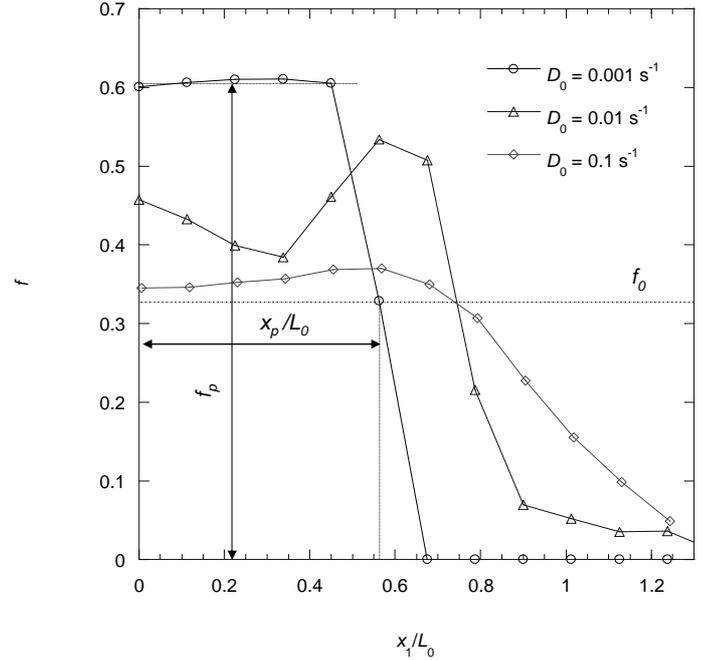
Figure 2: Evolution of the fibre content  $f$  along the normalised abscissa  $x_1/L_0$  at various initial strain rates  $D_0$  (compression elongation  $\lambda_f = 0.4$ , initial sample length  $L_0 = 80$  mm).
