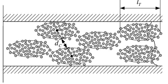
Fig. 2 Flow front of resin between fiber tows
