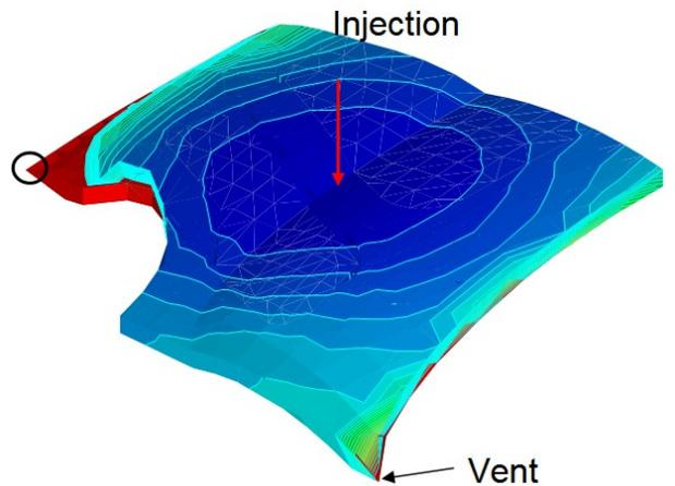
(b) Resin and air flow with the vent pressure applied at the air vent
