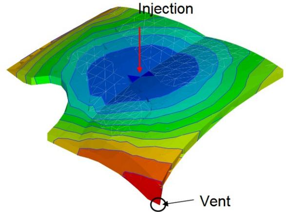
(a) Resin flow with the vent pressure applied at the flow front
