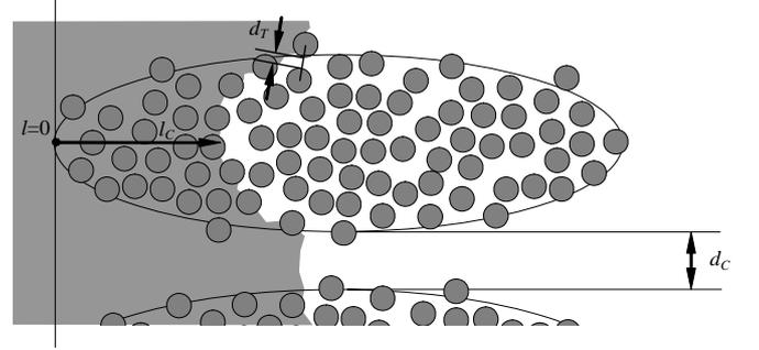
Fig. 3 Flow front of resin within a fiber tow
