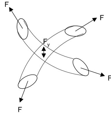
Figure 2: Inter-yarn force  $F_y$  due to yarn tension F
