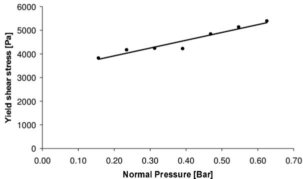
Fig. 6. Influence of the normal pressure on the yield shear stress at a temperature of 195°C and a velocity of 25 mm/min
