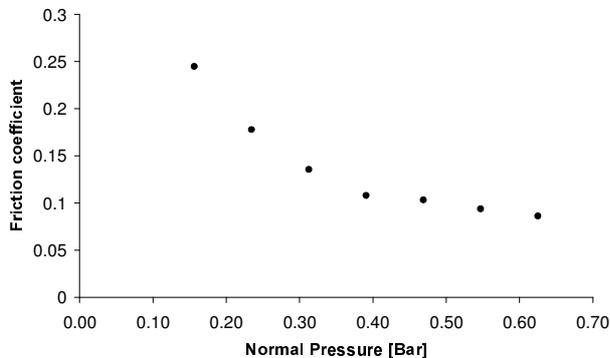
Fig. 7. Influence of the normal pressure on the friction coefficient
