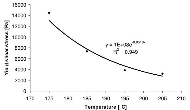
Fig. 5. Temperature dependence of the yield shear stress at a velocity of 25 mm/min and a normal pressure of 0.16 bar
