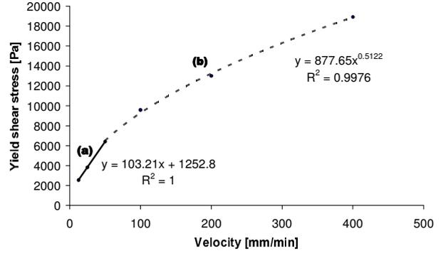
Fig. 4. Yield shear stress versus velocity at a temperature of 195°C and a normal pressure of 0.16 bar
