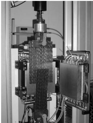
Fig. 1. Set-up for interply shear tests
