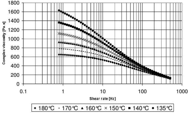
Fig. 3. Flow curves for PP at different temperatures
